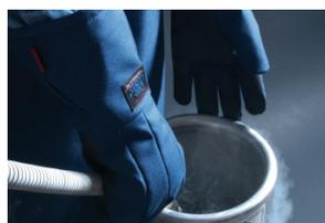
**5** Cryo gloves protect your hands and prevent frost bites when handling samples which are stored at down to -160 °C.
