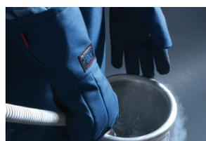
**6** Cryo gloves protect your hands and prevent frost bites when handling samples which are stored at down to -160 °C
